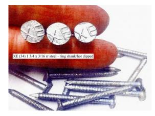
This XE, like the one listed earlier was used by Osmose when treating poles owned by Xcel Energy Corp. I believe this nail predates the (15) XE nail. This one is type (34) 1  $3/4 \times 3/16$  and R steel and has a ring shank the entire length of the shank. It is "hot dipped" in molten zinc, the old fashioned way.
