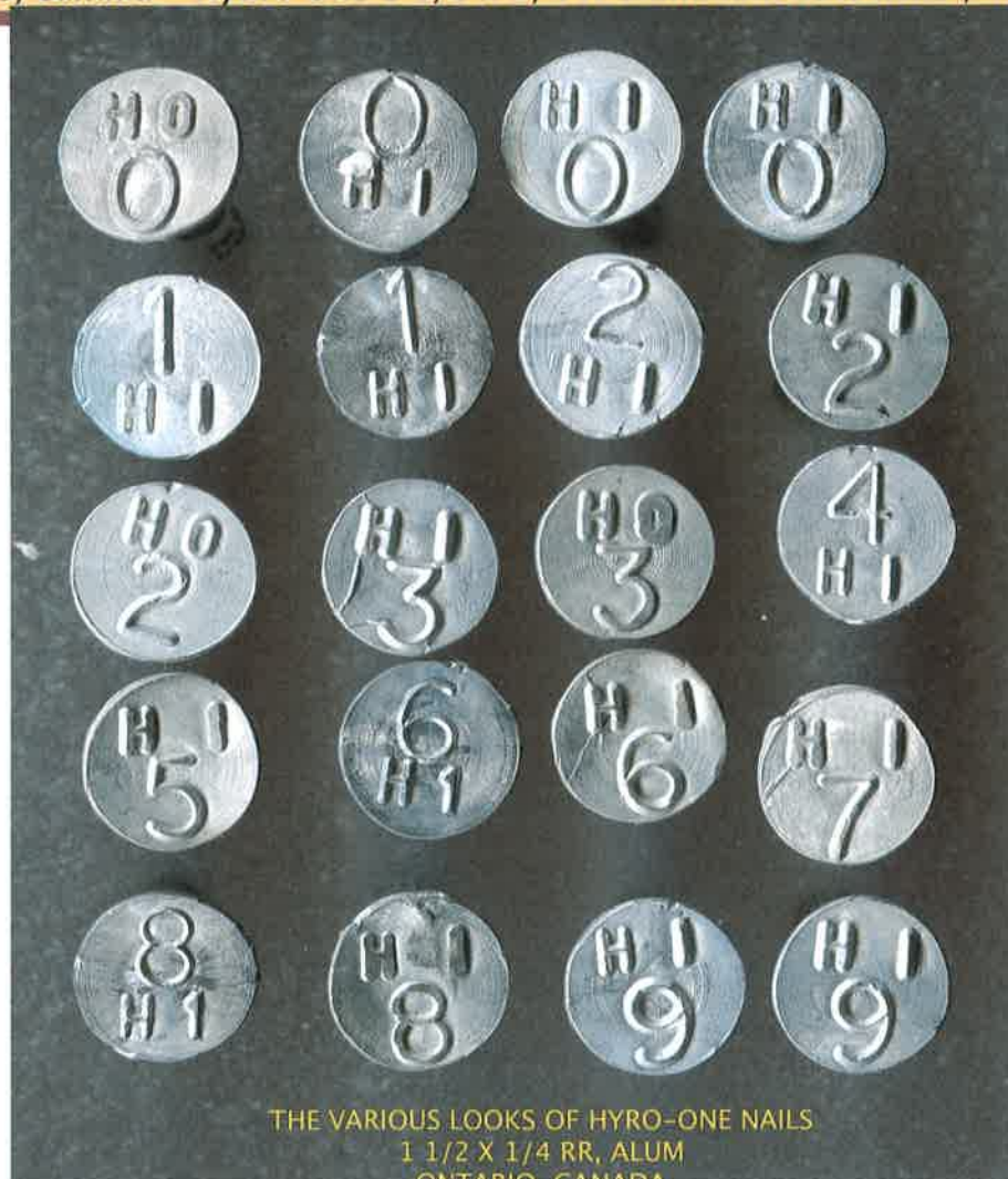
Ontario, Canada – Hydro One 1 1/2 x 1/4 rr aluminum date nails / with dies
