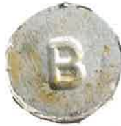
B ( ) 1 1/2 x 1/4 ri alum. Borate treatment nail. BPB treated ties used by Norfolk So. RR
