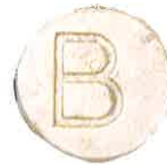
B ( ) 1 1/2 x 1/4 ri alum. Borate treatment nail. Found in ties
