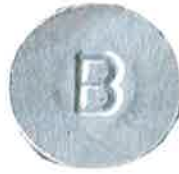
B ( ) 1 1/2 x 1/4 ri alum. Borate treatment nail used by BPB in ties
