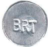
BRT ( ) 1 1/2 x 1/4 ri alum. Borate treatment nail used by Stella Jones for treated ties
