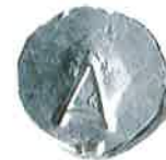
1 1/2 X 1/4 rnd l alum Clendenin nail stamped by Premax. Used by Nova Scotia Power to Number buildings etc.
