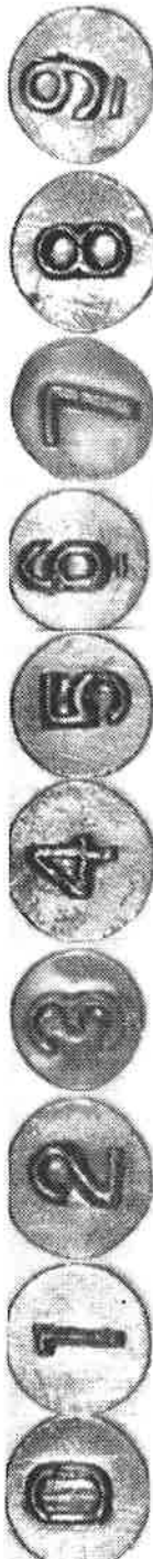
Set #10. 2 1/2 × 1/4 rnd R stl (07) Oklahoma Gas & Electric and Detroit Edison Co. Used to number poles. Georgia RR, used to number switches. Boston & Maine RR, to number ties in a test section in North Conroy, NH. See also Set #18.
