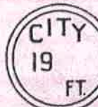
Fig. 5 With spaces left for completing the date and stamping pole heights.
